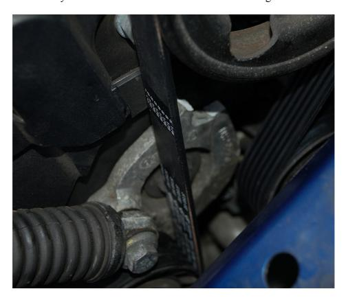
... all is not necessarily lost. Get the belt in position, pop your hand under the belt tensioning pulley and imagine your child is trapped underneath.
